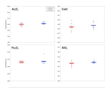
**Figure 2:** Graphical display of XRF analysis of concentration of  $Al_2O_3$ , CaO,  $Fe_2O_3$  and SiO<sub>2</sub> after sample preparation in the HP-MP 2 (red) and HP-MP 3 (blue).
