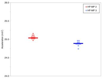
Figure 3: Graphical display of the acceleration values obtained from the ten grinding cycles obtained within the HP-MP 2 (red) and the HP-MP 3 (blue).
