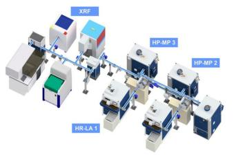
**Figure 1:** This graph displays the layout of the quality control laboratory of a German cement plant. The samples are pneumatically sent within air tube carriers from the plant to the laboratory. The carrier arrive in the laboratory station HR-LA where there are unpacked and dosed into cups which are then transported to the HP-MP for sample preparation.
