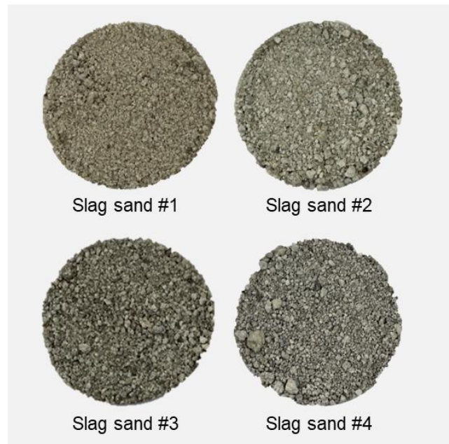
Figure 1: Photographs of the four different slag sand types examined in this study.
