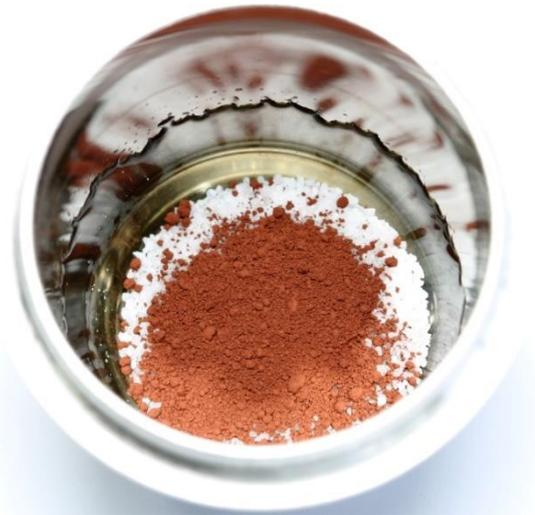
**Figure 2:** Protection wall within a new crucible with a polished inside. The protection wall is half as high as the crucible. The oxidizing agent (white) and the sample material (brown) can safely be oxidized without contact to the platinum.
