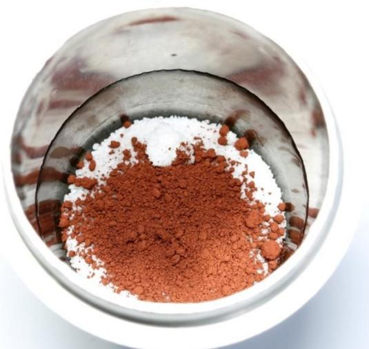
**Figure 3:** Protection wall within a used crucible. The protection wall is half as high as the crucible but more sharply delineated compared to Figure 2.
