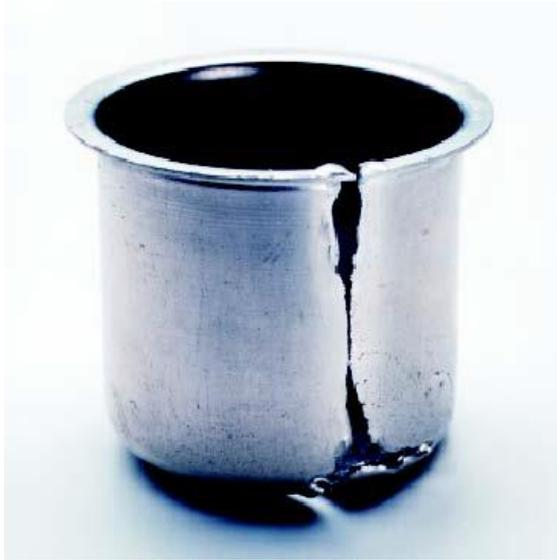
**Figure 1:** Melting of a platinum crucible after contact with SiC at high temperatures (LUPTON et al. 1995).
