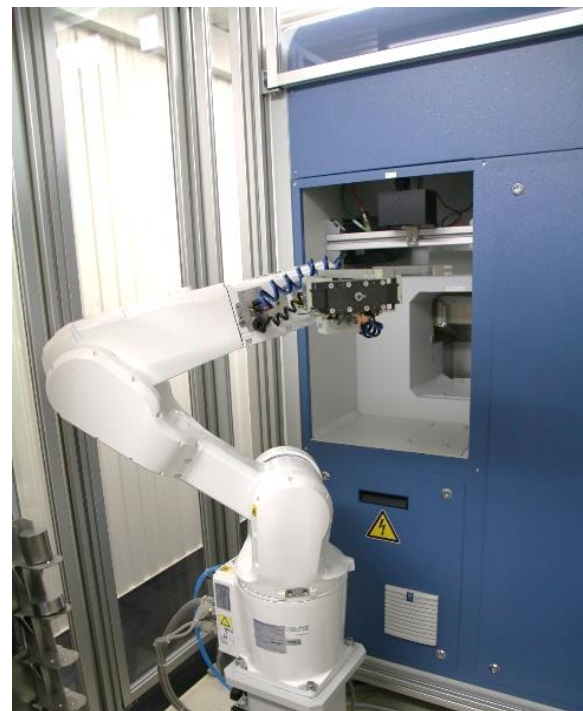
Figure 4: Rear opening of the HS-F 1000 for robot access into the milling machine including camera system for sample inspection
