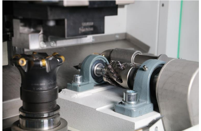
Figure 1: The module for production of granular chips is fully integrated into the milling machine HS-F 1000. After removal of the uppermost layer by the face-milling cutter the sample is transported to the module.
