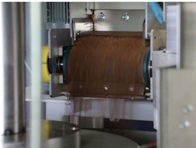
Figure 2: Photo showing the material stream of iron ore on the conveyor belt above the division drum.
