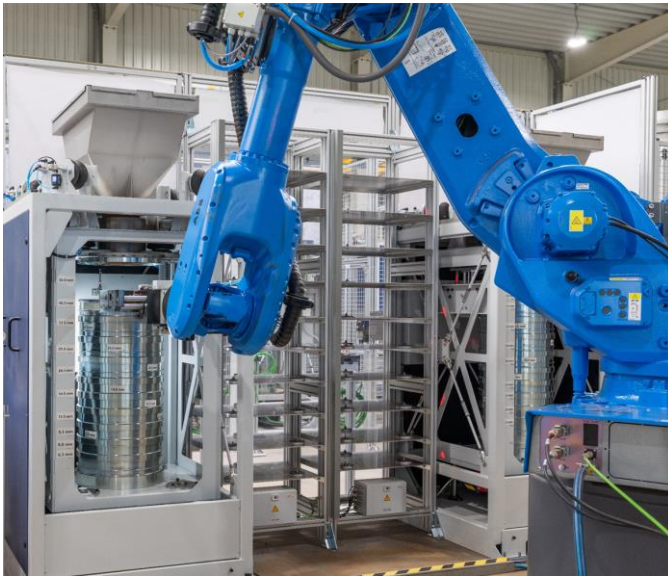
Figure 1: HP-SST integrated in a robot cell- photo shows HP-SST during unloading of sieves.
