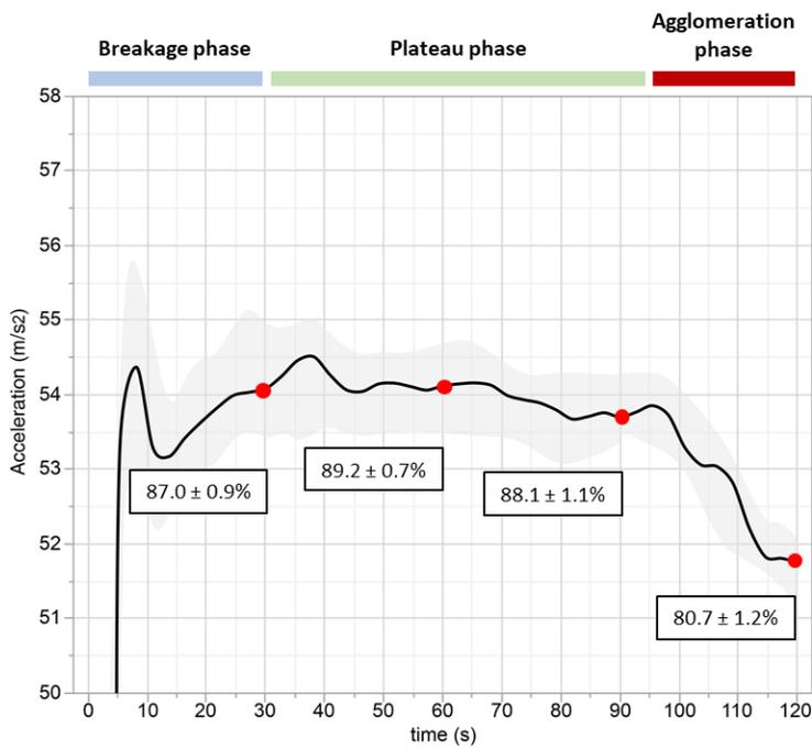
**Figure 4:** Display of the average acceleration curve built from single trials during grinding of clinker. Within the boxes the % portion ( $\pm$  SD) of particles below  $45 \mu\text{m}$  is indicated. The different phases are clearly distinguishable based on the acceleration curve.
