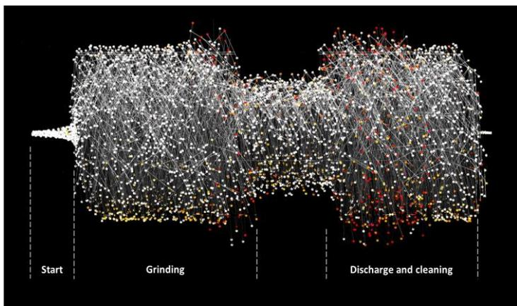
**Figure 1:** Graphical display of acceleration values in *x*- and *y*- direction over time. In this example various stages of a typical grinding cycle are shown including start of the grinding process, the grinding itself as well as discharge of the material from the grinding vessel and cleaning of the grinding vessel. This application note focuses on the detailed assessment of the grinding phase.
