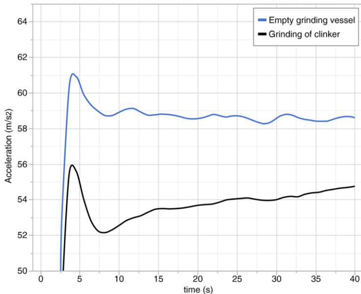
**Figure 2:** Comparison of acceleration curve during motion of an empty grinding vessel (blue line) and during grinding of clinker (black line).
