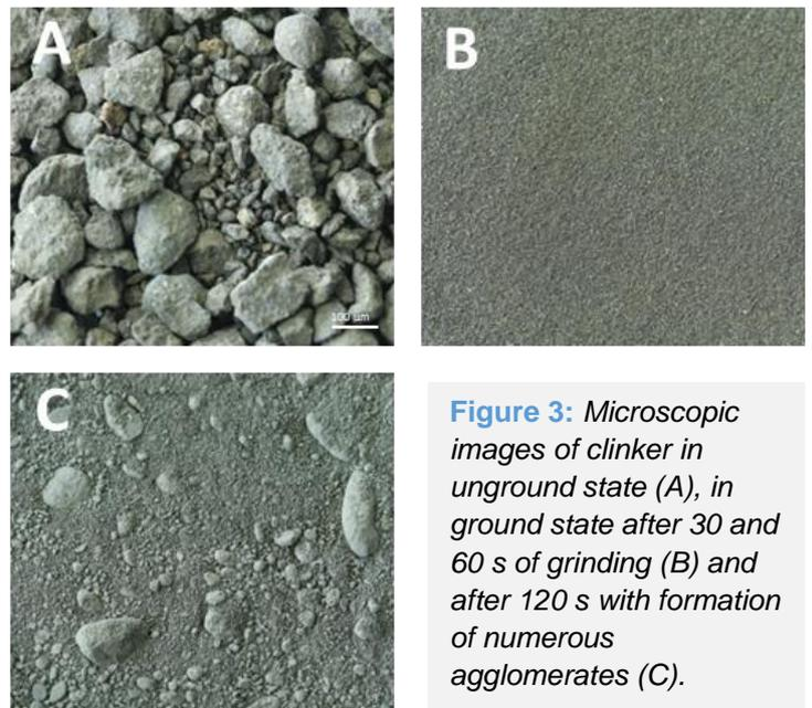
**Figure 3:** Microscopic images of clinker in unground state (A), in ground state after 30 and 60 s of grinding (B) and after 120 s with formation of numerous agglomerates (C).
