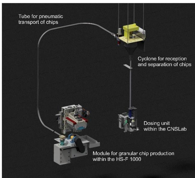
**Figure 1:** Basic experimental setup with chip transport from the HS-F 1000 to the receiving cup in the dosing unit of the CNSLab.
