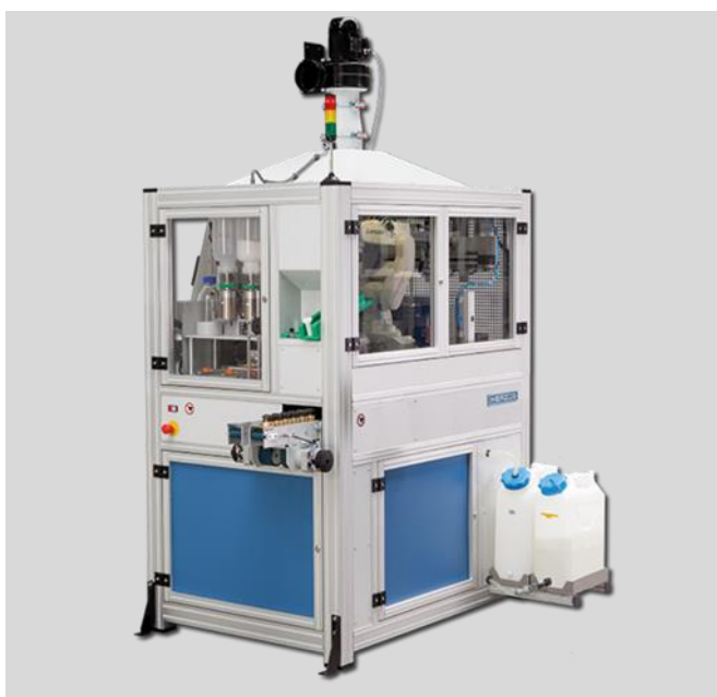
Figure 1: Automatic high-frequency fusion system model HAG-HF for XRF sample preparation. The machine also includes the dosing unit used for this study.
