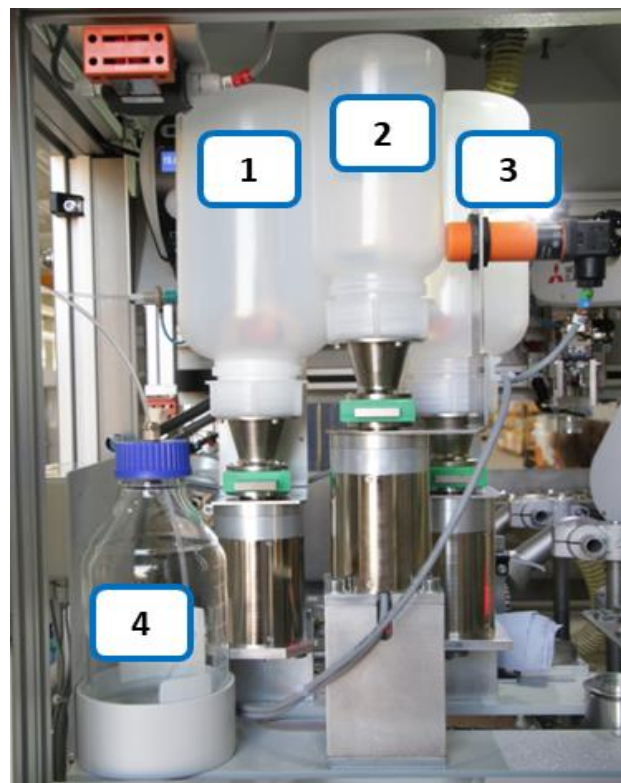
Figure 1: Detail photograph of the dosing unit of the HAG-HF with bins for (1) internal standard, (2) oxidizer, (3) borate flux, (4) liquid dosing of non-wetting agent.
