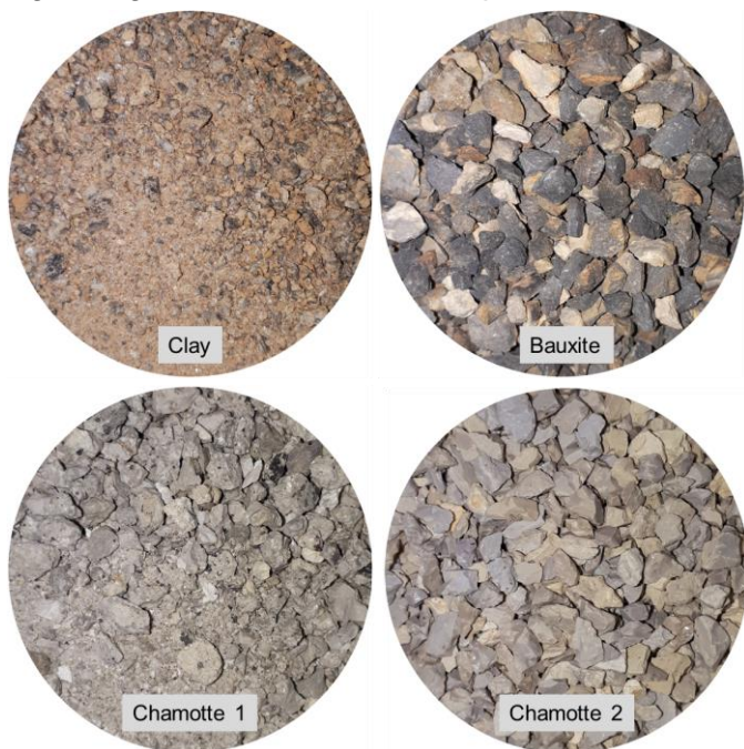
Figure 1: Photographs of four raw materials used for production of refractories. For this application note, we assessed the grindability of clay, bauxite and two types of chamotte.
