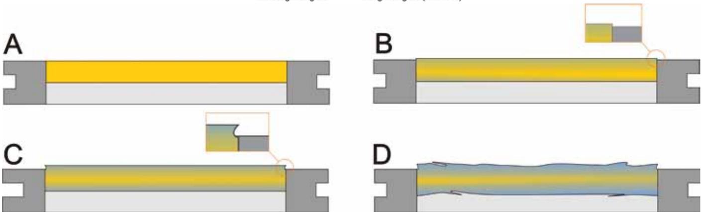
Fig.3: Schematic illustration of the moisture uptake of pressed pellets of lime after sample preparation without grinding aid.
