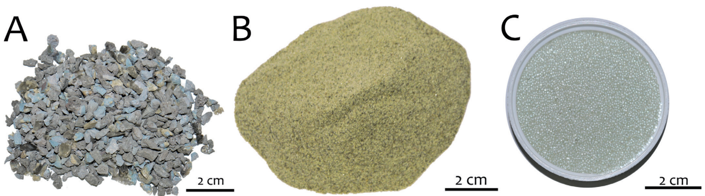
Fig. 2: Overview of the material used for the artificial sample used for the splitting test. (A) slag (>2 mm), (B) phosphate concentrate (<500 \mu\text{m} ), (C) glass spheres (1 mm – 0.75mm)
