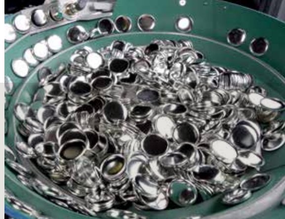
Input of inlays by vibratory unit
