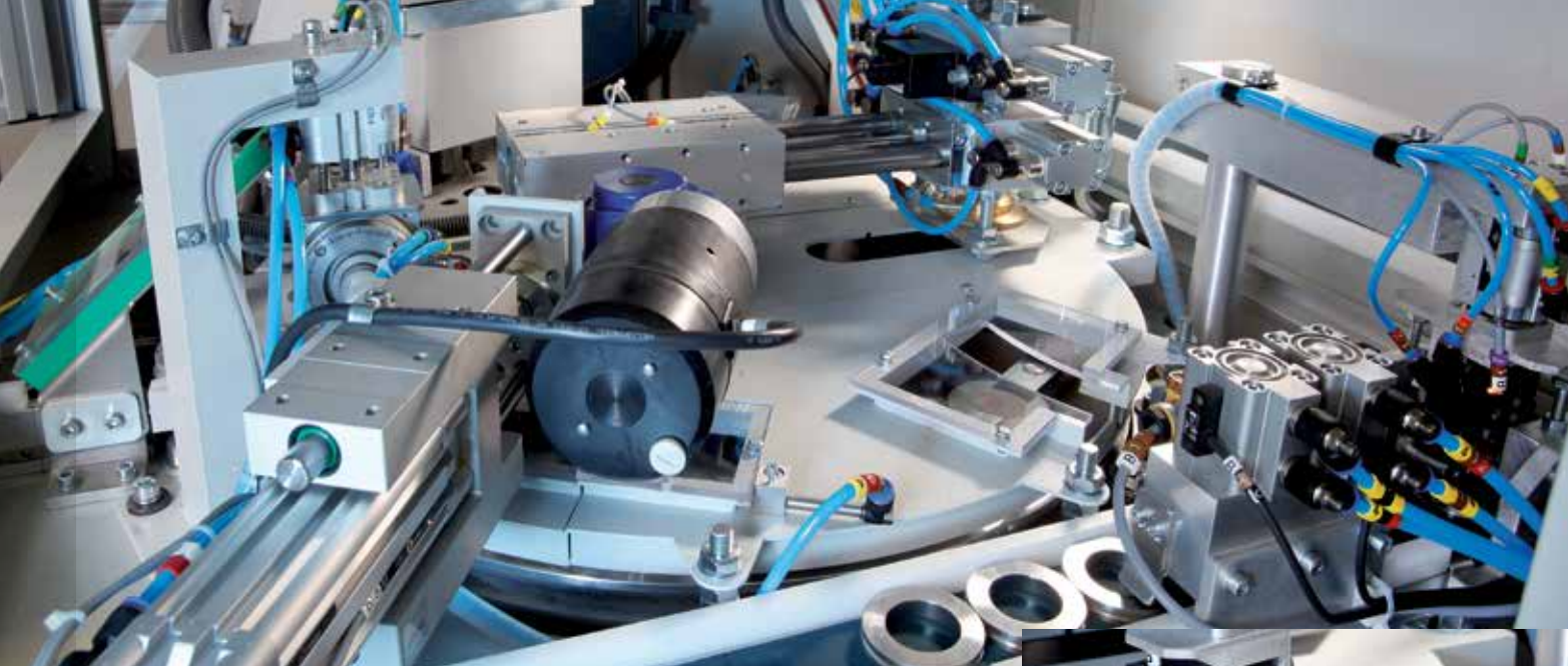
Interior of HP-PD6 with cleaning equipment (front left) and ring input (front right)
