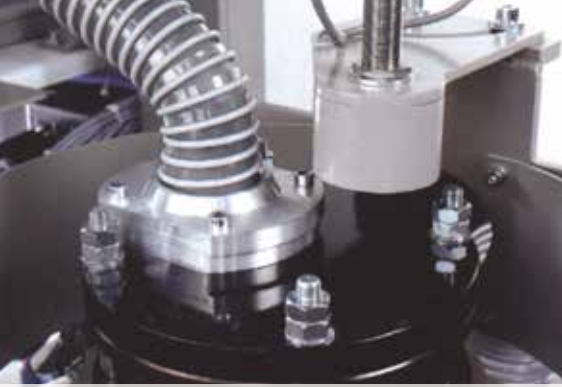
Temperature sensors with cooling of the pulverising vessel
