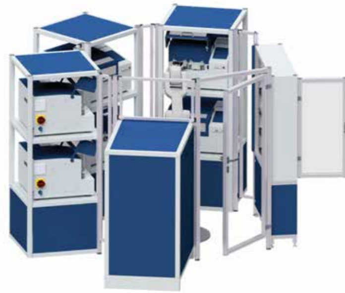
Integration of the HP-SKM in automated laboratories: handling of grinding vessels using a multi-axis robot
